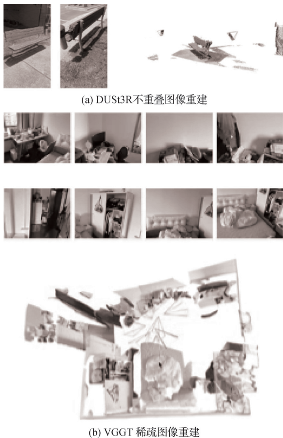
图 4 前馈式重建稀疏视角/欠定条件重建 Fig. 4 Feed-forward reconstruction for sparse-view/ underdetermined-condition reconstruction (a) DUST3R non-overlapping image reconstruction; (b) VGGT sparse image reconstruction)
